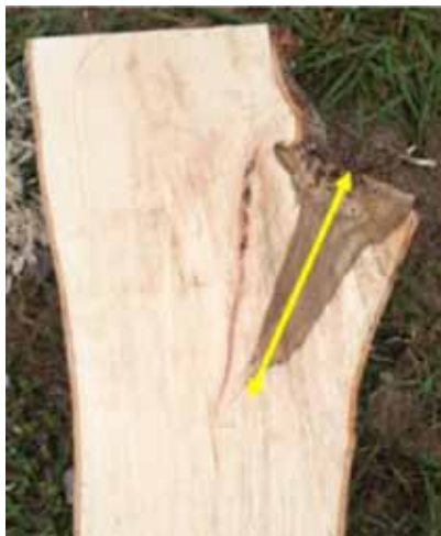
Figure 3. Trunk sections were dissected along the midpoint of the trunk-branch union to measure the extent of discolored wood within the branch protection zone. Arrow shows the depth of discoloration. Area of discoloration was also measured.
