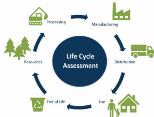
Life Cycle Assessment diagram. LCA is an international standard that captures the environmental impact of a given product from birth to death. USDA Forest Service image.
